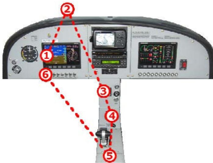
"Engine Failure After Takeoff" checklist flow
