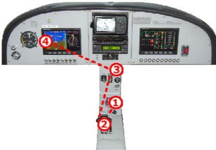
“Engine Fire In Flight” checklist flow
